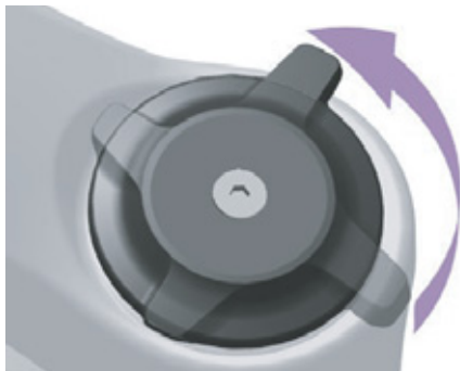
Figure 79: Changing compression adjuster to a softer setting
