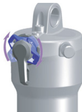
Figure 71: Changing compression adjuster to a harder setting
