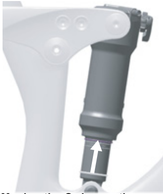
Figure 60: Moving the O-ring on the rear frame damper
