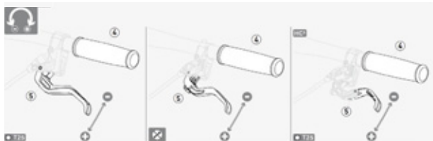
Figure 51: Adjusting the grip distance on a Magura disc brake lever
