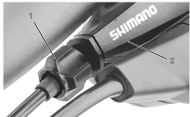
Figure 86: Adjusting sleeve (1) for the single-cable, cable-operated gear shift with shifter housing (2), example
