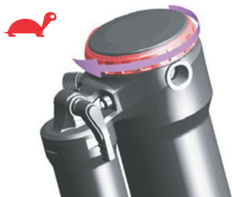
Figure 98: Turning rebound damper towards tortoise symbol
