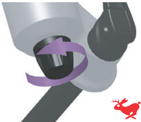
Figure 92: Turning rebound damper towards hare symbol
