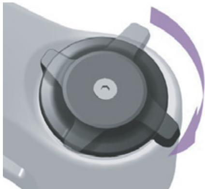
Figure 78: Changing compression adjuster to a harder setting
