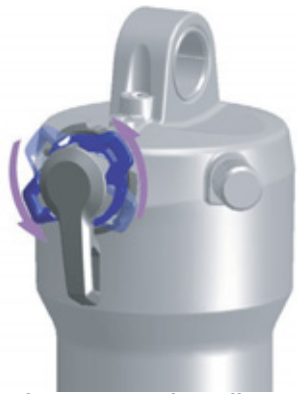
Figure 104: Changing compression adjuster to a softer setting
