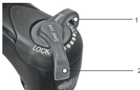
Figure 77: Suntour compression adjuster in open (1) and closed (2) position
