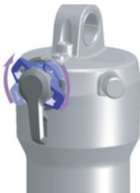
Figure 102: Changing compression adjuster to a harder setting
